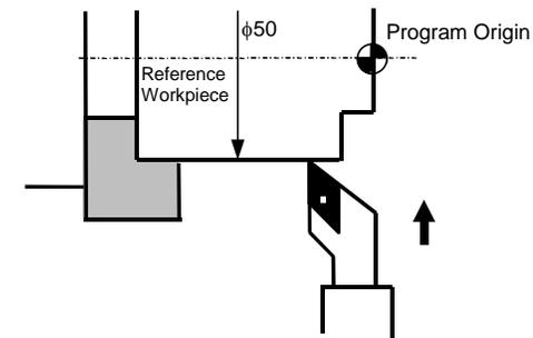
Enter the distance from the rotational center of the turning spindle (X), which is **a diameter value**, by using numeric keys. >> In case of the above figure, enter "50."
