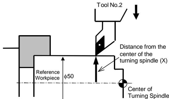
Enter the distance from the rotational center of the turning spindle (X), which is **a radius value**, by using numeric keys. >> In case of the above figure, enter "25."
