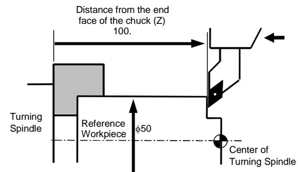
Enter **the distance from the end face of the chuck (Z)** by using numeric keys. >> In case of the above figure, enter "100."
