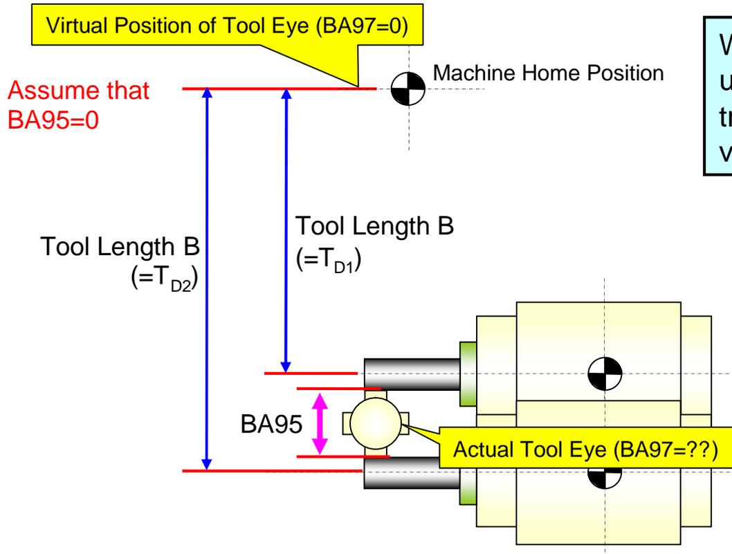
When the tool length B is measured under the condition that BA95 = 0, the true value of BA95 is included in T<sub>D2</sub> value.
