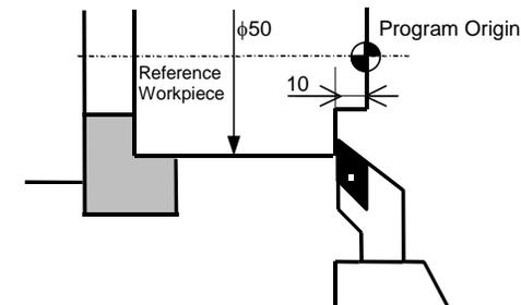
Set **the Z-coordinate value of the tool tip position to the program origin**. >> In case of the above figure, set "-10."
