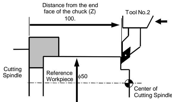
Enter **the distance from the end face of the chuck (Z)** by using numeric keys. >> In case of the above figure, enter "100."
