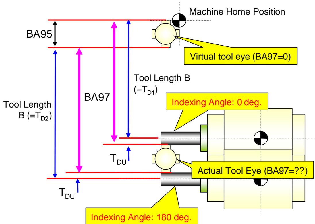
When the tool length B is measured under the condition that BA95 = 0, the true value of BA97 is included in  $T_{D1}$  and  $T_{D2}$  values.
