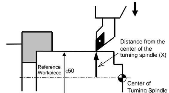
Enter the distance from the rotational center of the turning spindle (X), which is **a radius value**, by using numeric keys. >> In case of the above figure, enter "25."
