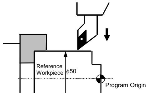
Set the X-coordinate value of the tool tip position to the program origin, which is **a diameter value**. >> In case of the above figure, set "50."
