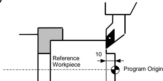
Set **the Z-coordinate value of the tool tip position to the program origin**. >> In case of the above figure, set "-10."
