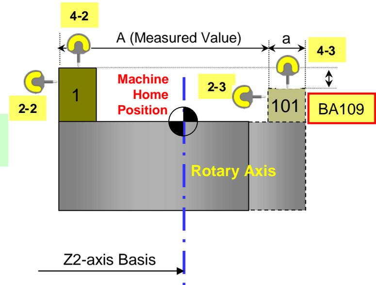
**NOTE)** BA110: Parameter to compensate the misalignment between the machine home position and the rotational center.
