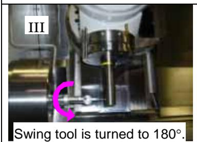
(2) Adjustment of RS12 (Measurement is carried out on the 2nd spindle under the condition of the Y-axis compensated and the B-axis at  $90^\circ$ .)
