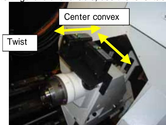
The W-axial level is measured.
