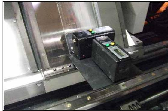
The Z-axial level is measured.
