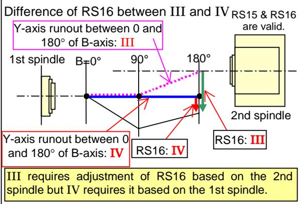
**(4) Parallelism of milling test bar**
